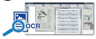
Scan2OCR is an optional software function which allows the user to scan in job mode and to OCR the entire page or multiple pages scanned, using multipage PDF mode. The OCR process runs in the background so that you can continue scanning subsequent pages in the job. This function is useful when scanning complete source material such as books, legal files and other multipage documents for which the operator wants all of the text OCRed.
